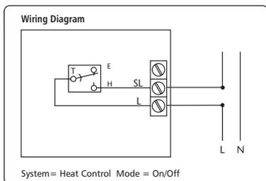
There are only two electrical connections required to the ST320, and these connections should be made to the terminal block inside the thermostat. No Earth connection is required for the correct and safe operation of the ST320, but a parking terminal is provided to connect an Earth wire if one is present. These connections are shown in the drawing and table below:
