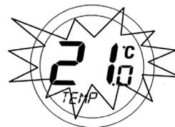
When the set temperature is flashing, press the Touch Ring and move your finger clockwise to increase the set temperature, or anti-clockwise to decrease the set temperature. Press OK at any time to confirm the selection. Note that the set temperature display will not flash while being adjusted – this is normal and the display will start to flash again approximately 0.5 seconds after the Touch Ring is released.
