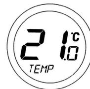
This will display the current set temperature. The set temperature will be displayed for two seconds before the LCD changes to display the room temperature again.
