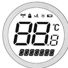
The display consists of a combination of symbols and alphanumeric displays. The top row is a set of status symbols, the centre row is used to indicate temperature (in Celsius), and the bottom row is an alphanumeric display for menu and status messages.
