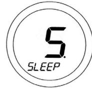
Pressing the OK Key at any time within the 5 seconds will cause the ST320 to immediately go into SLEEP mode, as will allowing the countdown to complete. Pressing the Arrow key will return the ST320 to the Menu display mode.
