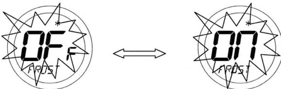
On entering the menu, use the Touch Ring to scroll to the preferred option (OFF or ON), and confirm the choice using the OK button. Use the Arrow key to return to the Menu Option display.
