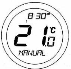
When the ST620 is operating in Manual Override mode, the LCD will display MANUAL instead of AUTO. The manual setting will remain in effect until the next programme time is reached, programme or clock settings are changed, an operating mode change is detected or the Manual Override mode is cancelled.
