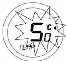
Use the Touch Ring to set the preferred temperature and confirm the choice using the OK button. Once the temperature setting is confirmed, the HOLIDAY mode will be activated. While in this mode the HOLIDAY mode indicator
