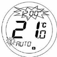
The ST620 time and day of the week settings are updated automatically every day (at 12:00 AM or 2:00 AM) by the use of a very accurate internal Radio Controlled Clock.
