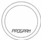
The Arrow key is not active when the ST620 is in NORMAL mode. To access the Menu screens, press the OK key twice. The first menu displayed is the PROGRAMME menu:
