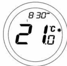
Pressing the Touch Ring will change the display to show the current temperature setting, but this setting cannot be adjusted while in this mode.
