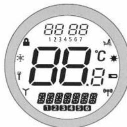
The display consists of a combination of symbols and alphanumeric displays. The top row is a time and day of the week indicator, the centre row is used to indicate temperature (in Celsius), and the bottom row is an alphanumeric display for menu and status messages. The symbols around the outside of the display are status indicators – an explanation of what these indicators mean is shown below.
