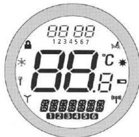
After 2 seconds the ST620 will then operate in NORMAL mode and display the current room temperature, with the RCC indicator flashing.
