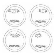
The hour setting will be the first setting that needs to be adjusted, and this will easily be seen because the 'hours' section of the time will be flashing. Using the Touch Ring, scroll up or down to adjust the hour to the required setting and then press the OK key to confirm.
