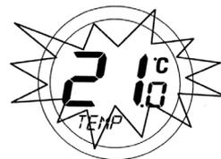
When the set temperature is flashing, press the Touch Ring and move your finger clockwise to increase the set temperature, or anti-clockwise to decrease the set temperature. Press OK at any time to confirm the selection. Note that the set temperature display will not flash while being adjusted – this is normal and the display will start to flash again approximately 0.5 seconds after the Touch Ring is released.
