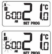
Pressing the SET key at any time when in programming mode will return the RT500 into **Normal** mode. Press the SELECT key to confirm the Day selection. Once this is set, the 'Hour' will flash to indicate that it is the selected item and is the next item to be adjusted:
